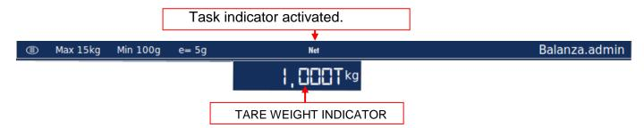
To eliminate the tare weight, retrieve the weight from the plate.
